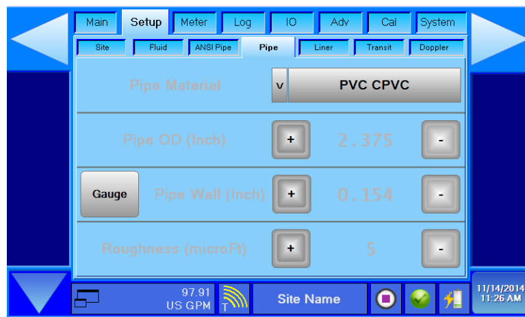
Figure 59: Pipe page from nominal entry
