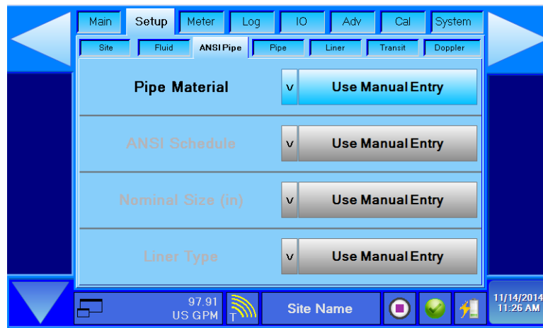
Figure 58: ANSI pipe page manual entry
