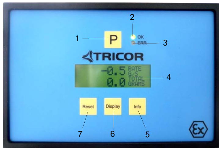
Fig. 6: Operating Elements of TCE80xx-L-Ex
