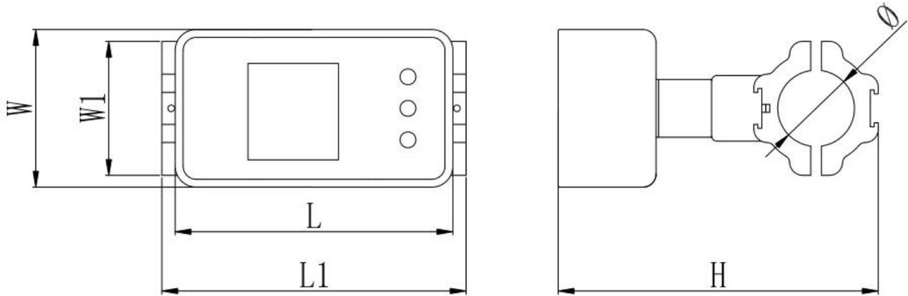
UltrasonicFlowmeter overall dimension drawing
